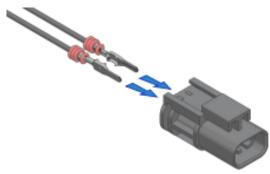
4. Install the red locking tab to secure the cables in place.
