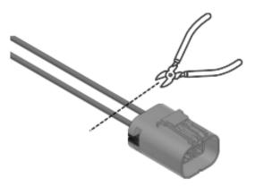
2. Remove ¼" (6mm) of cable shroud to reveal the wire core. Crimp the female spade connectors as shown.
