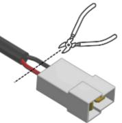
Slide the cables through the supplied rubber seals before removing ¼" (6mm) of shroud to reveal the wire core. Crimp the male spade connectors, noting the rubber seal position, as shown.
